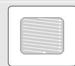
The progressive scanning method scans one full frame of video consecutively down the screen, line by line. As opposed to the interlaced scanning process by which a video image is drawn in a series of passes, you get an entire image drawn at one time.
